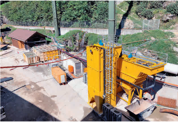
2 Piotta, impianto trattamento acque 60 l/s Piotta, water treatment plant 60 l/s
