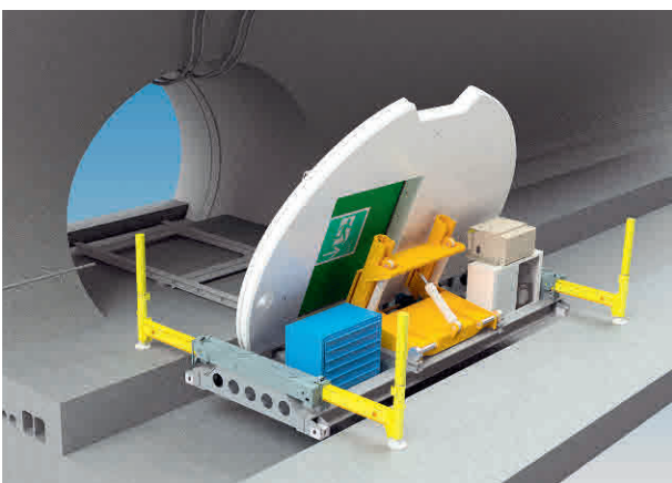
8 Manipulator am Einbauort Erector at the point of installation
