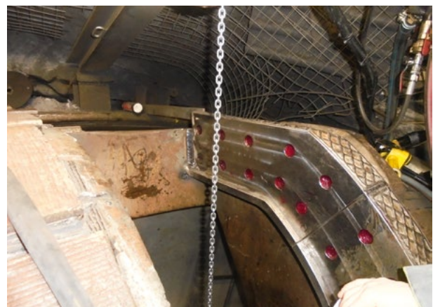
6 First welding chamber: replacement of anti-wear plates and replacement of supports of bucket tools
