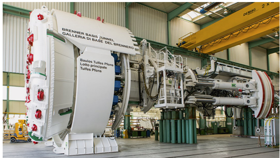
11 Gripper-TBM Gripper tunnel boring machine
