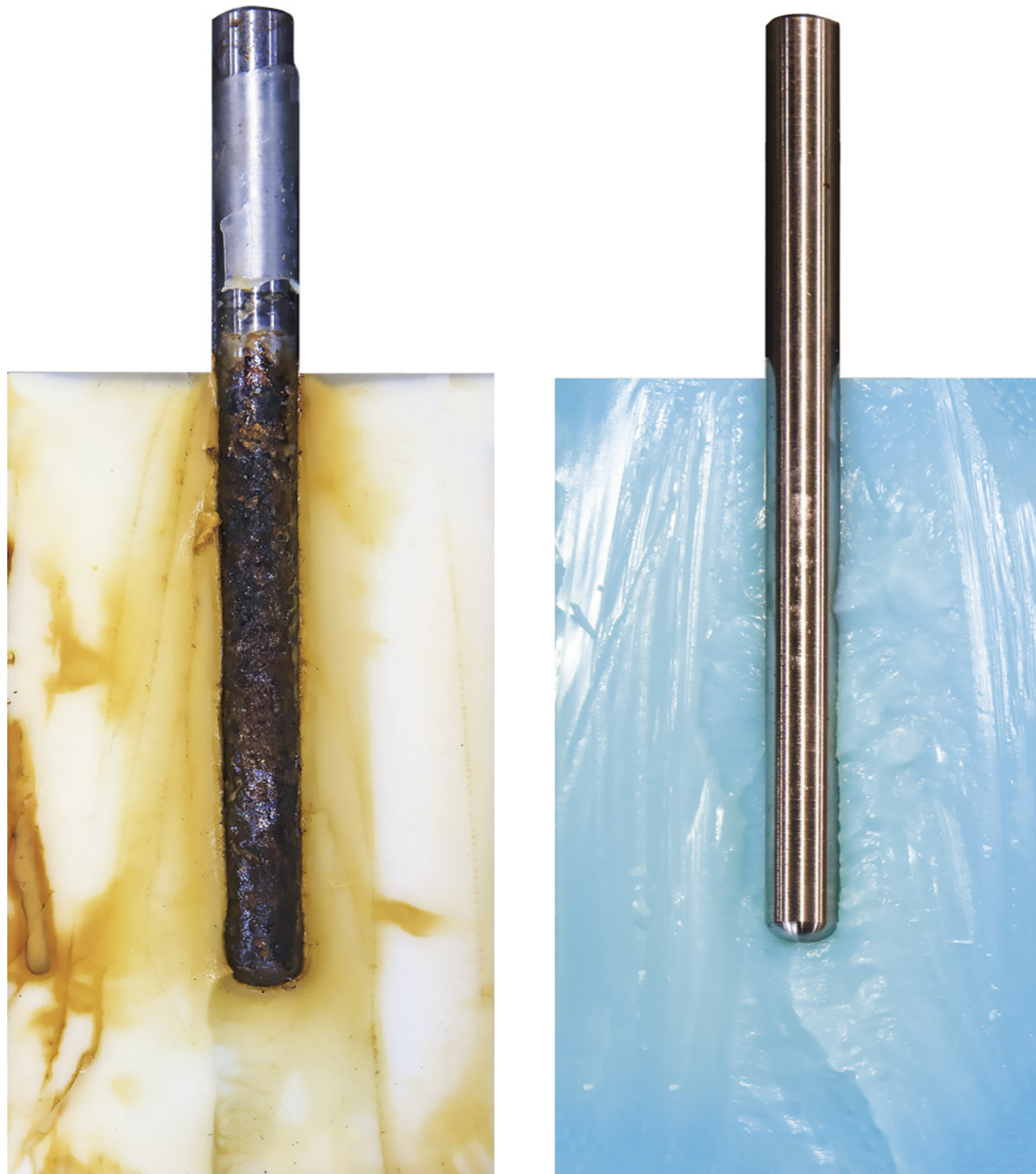
6 Lollipop Test. Conventional Acrylate vs Sika® Injection-307
