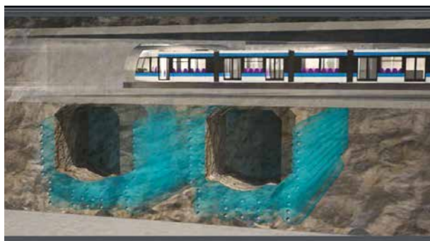
11 Cross section of Line C tunnels passing beneath the existing Line A station
