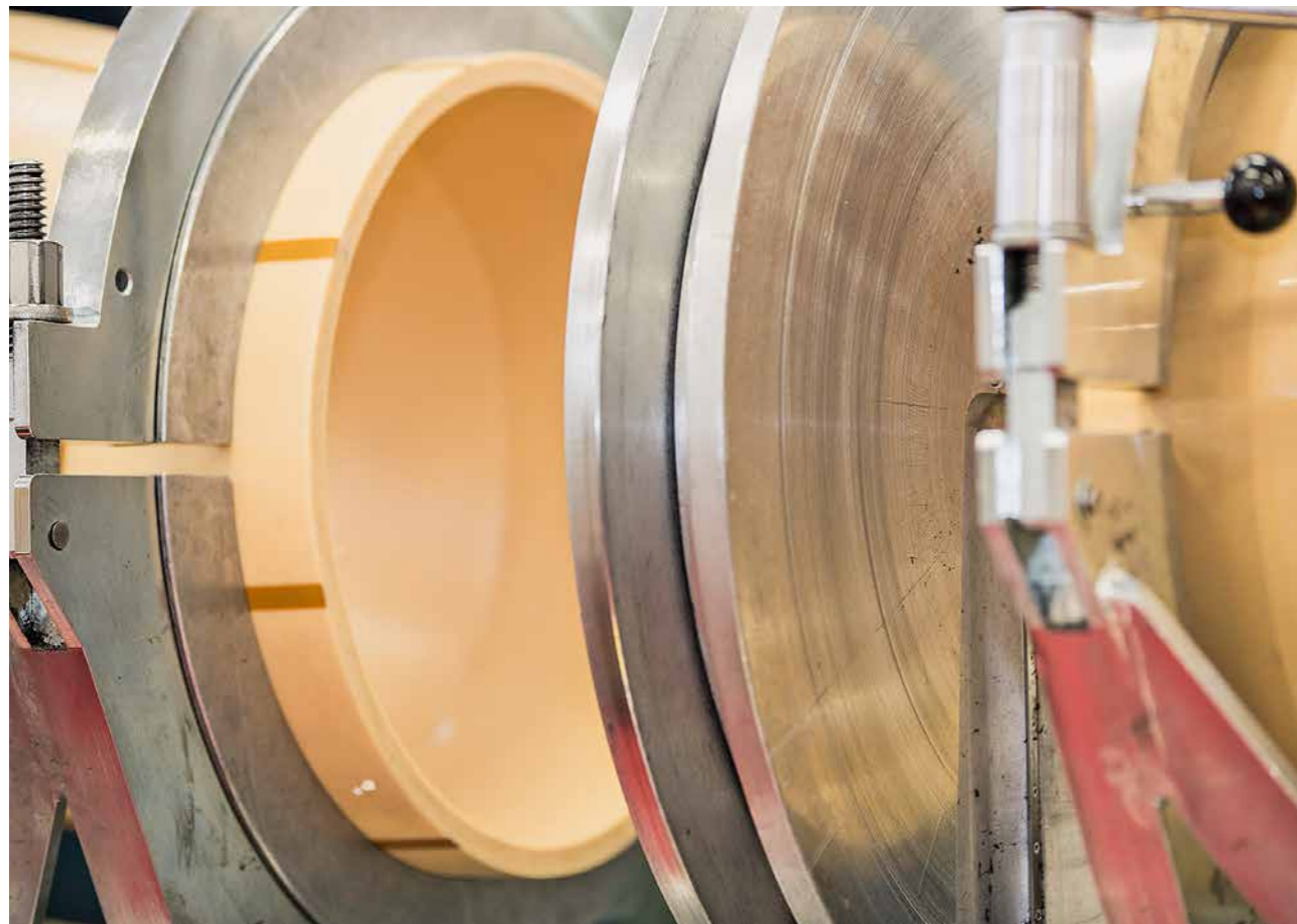
8 Spiegelschweissvorrichtung Mirror welding equipment
