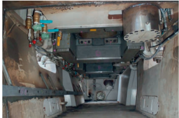
4 Hollow arm to access and replace cutting tools in atmospheric pressure
