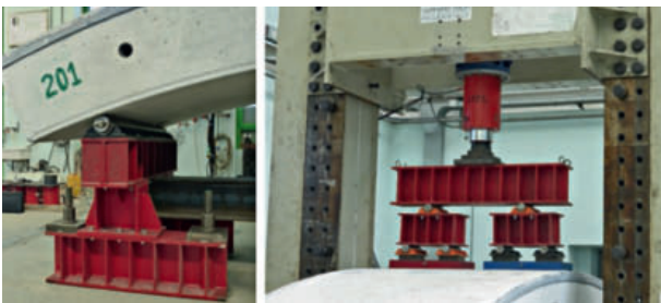
7 Bending test of one element of the lining
