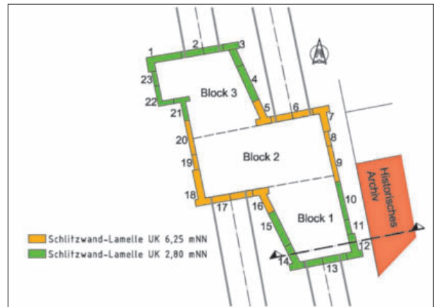
4 Lamelleneinteilung GWB Arrangement of panels in track crossover construction
