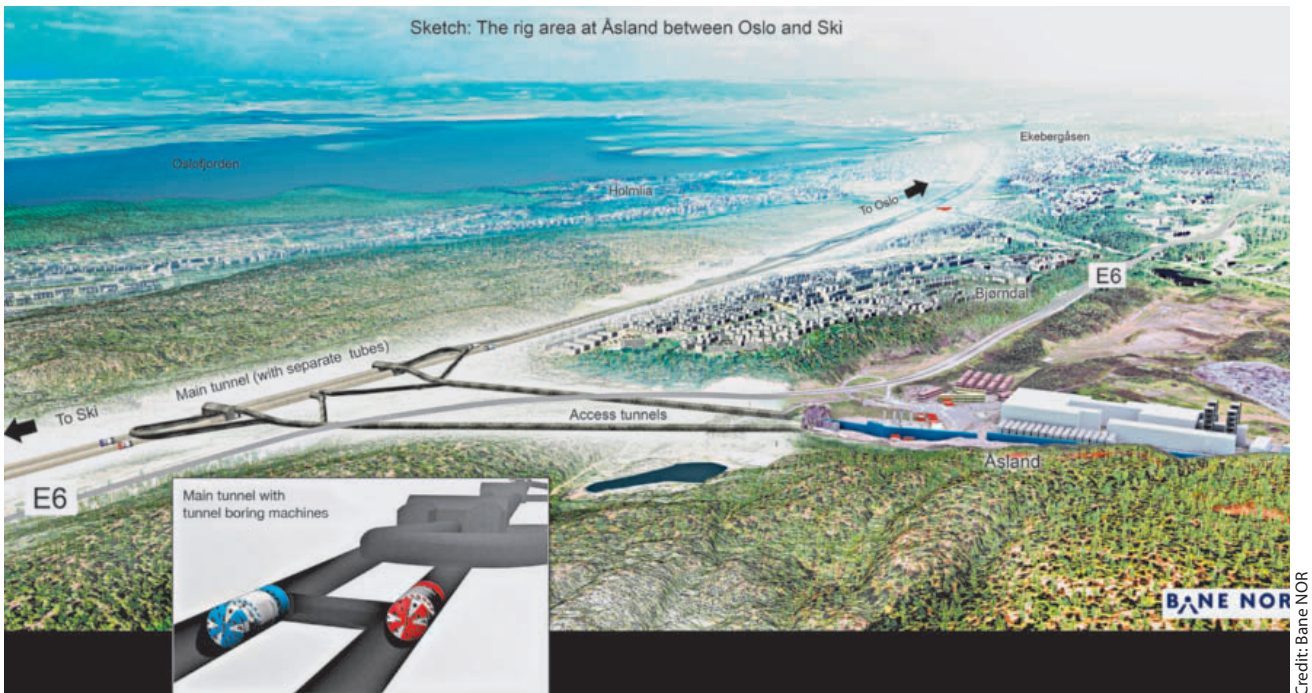
4 Four TBMs operating from one centrally located access point
