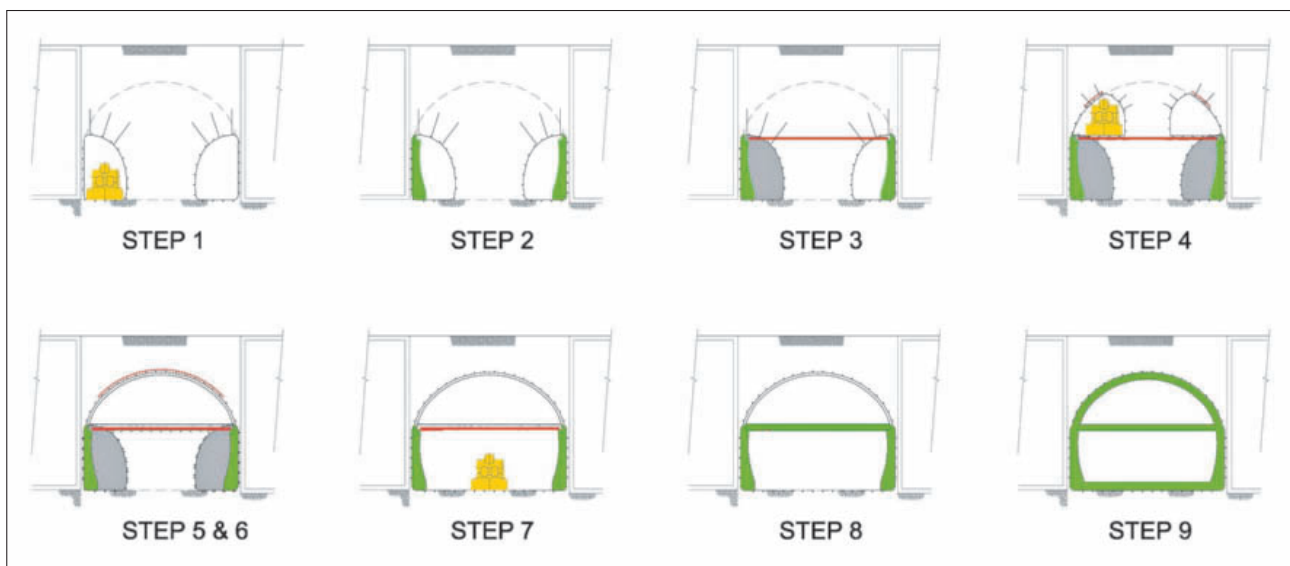
8 Excavation stages in Lyon and Parliament
