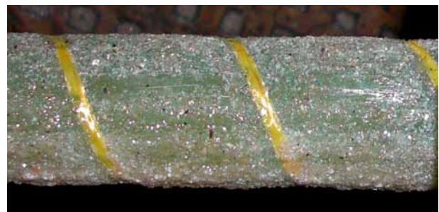
2 Glass fiber rod, with example of an enhanced bonding surface. A cm-scale boudinage is visible (Source: Sireg S.p.A.)
