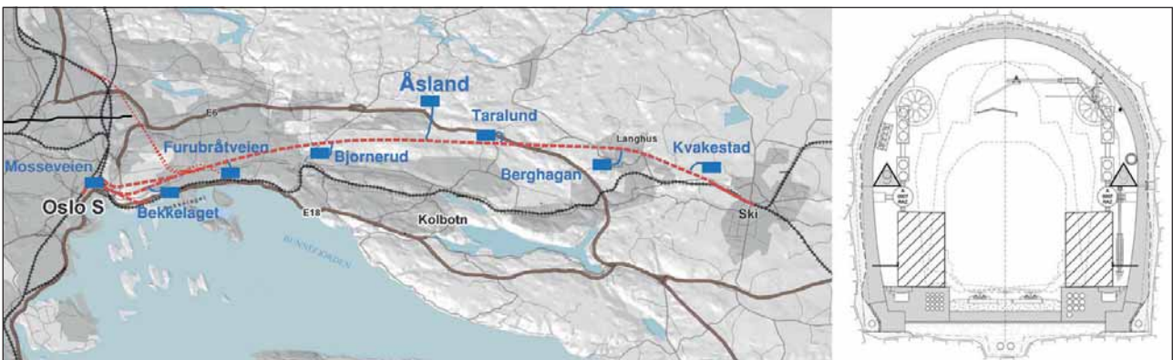
4 Drill & blast alternative: location of the intermediate points of attack [1] on the left and standard cross-section [8] on the right
