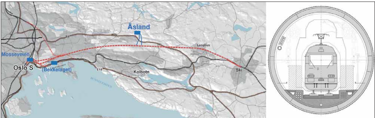
3 TBM alternative: location of the intermediate points of attack (for the TBM drives: Åsland) [1] on the left and standard cross-section [7] on the right
