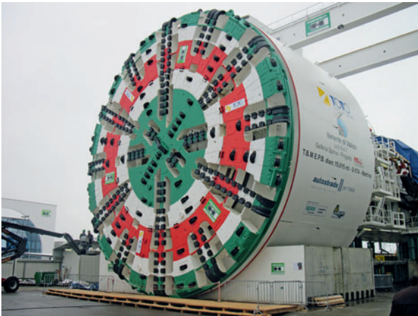
8a The Sparvo EPB TBM (named “Martina”)
