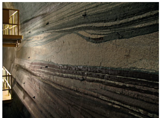
3 Gradueller Kontakt zwischen dem Queenston Tonstein und dem Thorold Sandstein [3] Gradual contact between laminated Queenston Shale and Thorold Sandstone [3]
