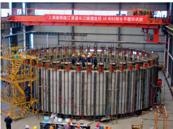
8 Set-up of full-scale test and loading system: testing site (left) and side view of loading system (right)
