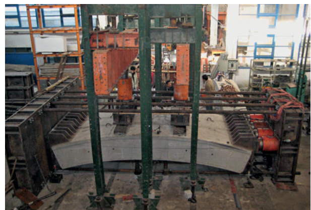
10 Segmental joint test [5]
