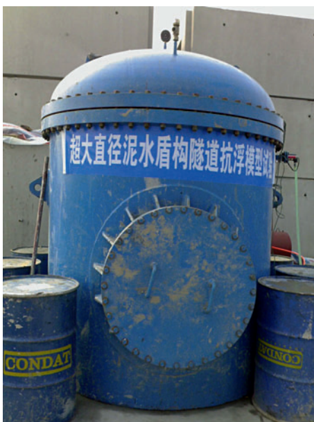
16 Experimental test of the relationship between the grouting and the up-heave of the tunnel: test equipment (left) and test design (right)
