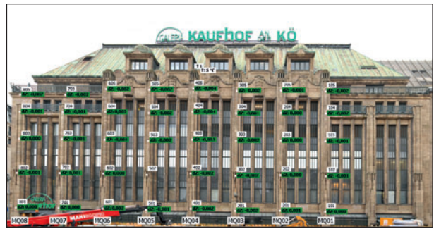
9 Fassadenmesssystem Facade measurement system
