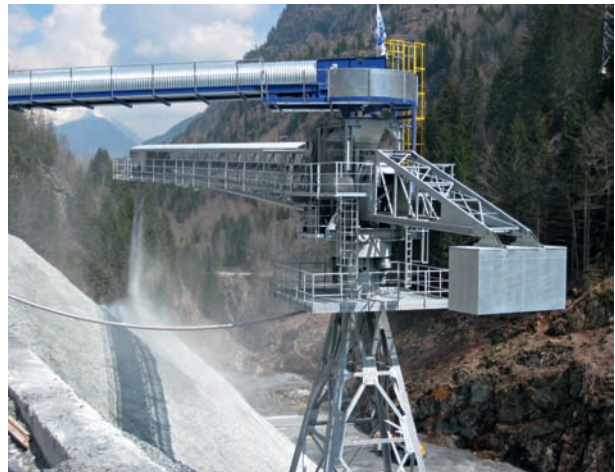
8 Schwenkabsetzer Nant de Drance (CH) Rotary stacker at Nant de Drance (CH)
