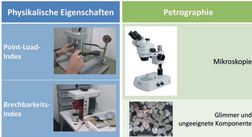
1 Tests on excavated material. Illustration of test methods.
