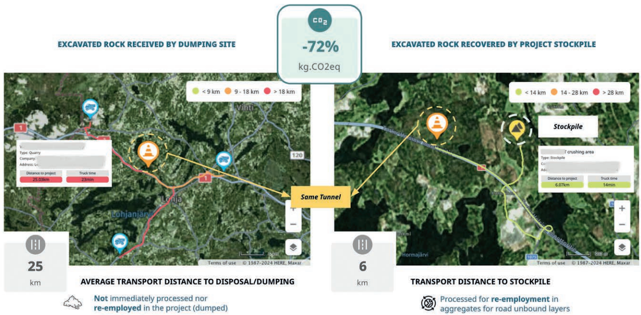
4 This figure shows an example of transporting the excavated material to a disposal site (left) versus a stockpile (right) and their effect on the CO 2 footprint.
