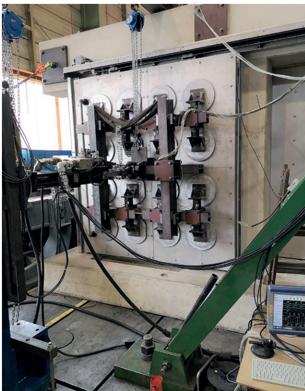
4 Long-term loading test for emergency exit doors
