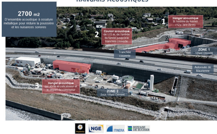
4 Aerial view of site installation with crushing hall and conveyor belt bridge over the river Arc
