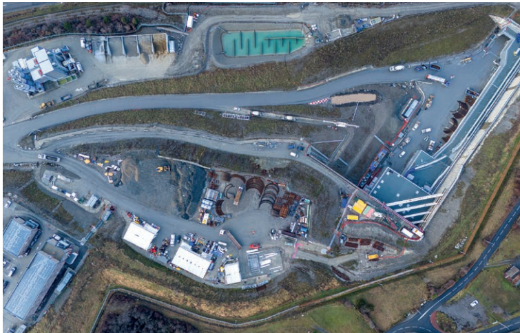
6 Aerial view of site installation with concrete plant, storage areas and preliminary cut
